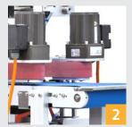
The split conveyor belt allows three or four sided labeling ensuring that products are sealed securely.
