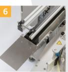
The 152C masters various mounting conditions and production environments. The conveyor belt is available with a width of 100 or 150 mm, at a length of 1,540 mm.
